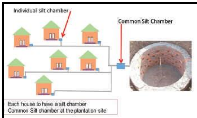
Figure 3.15 Community Leach Pit. Maximum number of Houses = 10. Quantity of Grey Water per day HH=300 Litres
