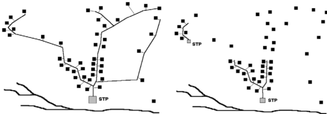
Figure 3.7 Concepts of Centralized (Left) and Decentralized (Right) Sewerage Systems. The squares represent houses or individual sources.
