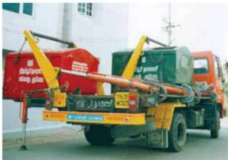
Fig. 1.11 Skip Truck (Dumper Placer) (Municipal solid waste management manual, Govt of India, 2014)
