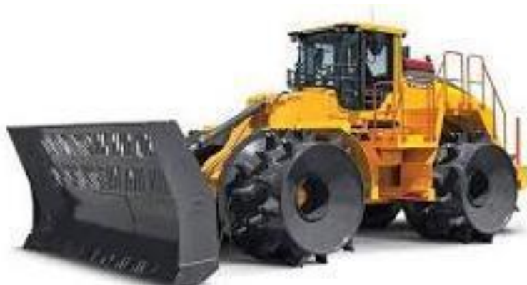
Fig 3.7 Landfill Compactor (Source: Challenges and opportunities associated with waste management in India. Sunil Kumar et al, Mar 2017. http://rsos.royalsocietypublishing.org/content/4/3/160764. )
