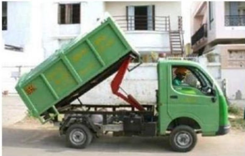
Fig. 1.6 Mini Truck with hydraulic container (Municipal solid waste management manual, Govt. of India, 2014)
