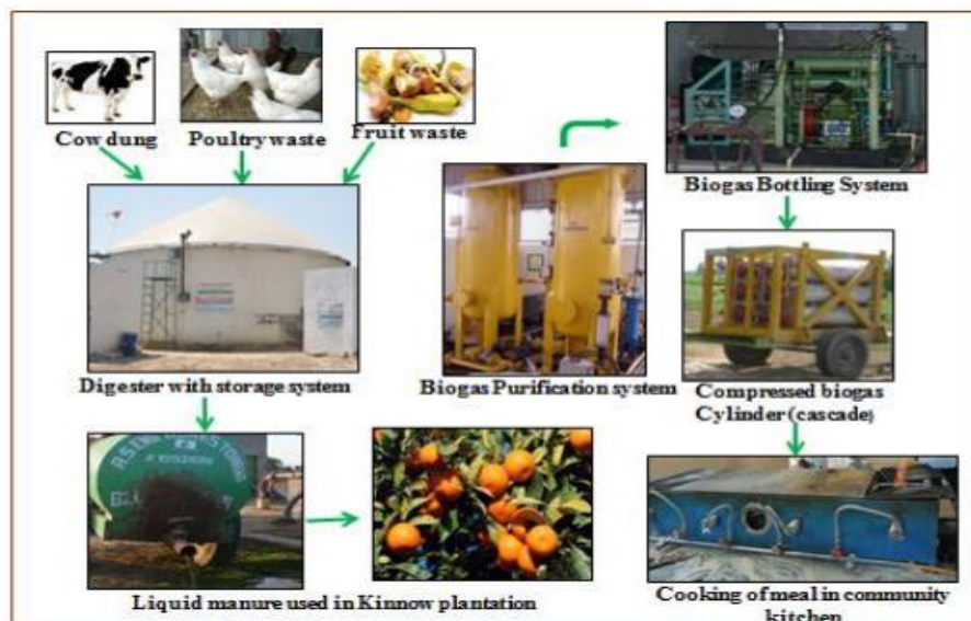
Fig 5.4 Bottled Biogas Manufacturing Process
