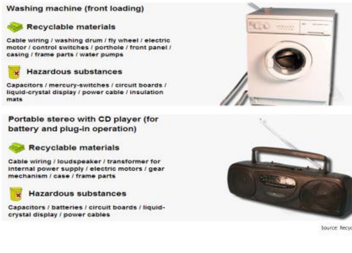
Fig2.4 Recyclable material and hazardous substances in a washing machine and a CD player
