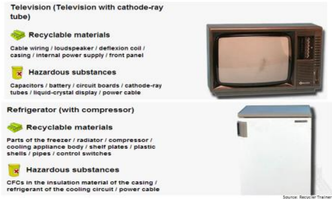
Fig2.3 Recyclable material and hazardous substances in a TV and refrigerator
