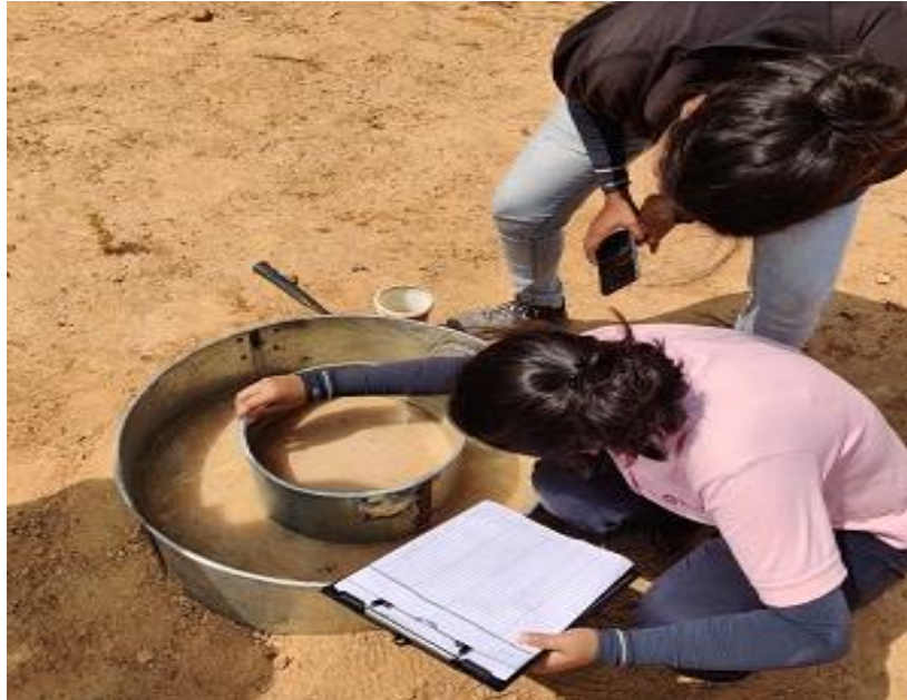
Soil Percolation Test Done by Geologists of Geovale Services
