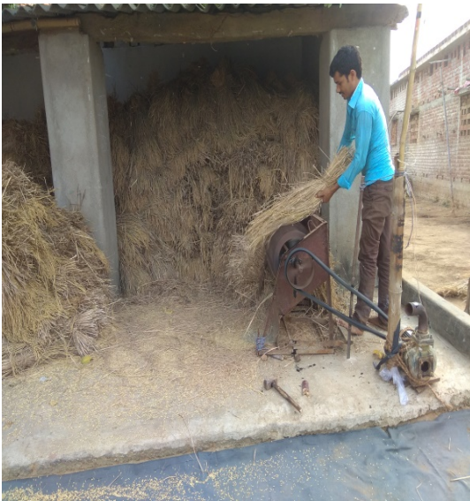
Anil Ji using his paddy separation machine after his harvest
